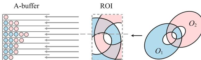
Fig. 5. Surface buffering for complicated collisions
