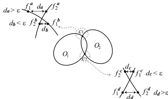
Fig. 4. PCS generation using the distance threshold
